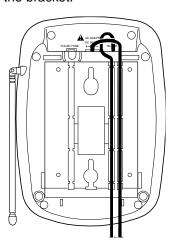
7. Align the keyhole slots with the mounting screws and slide the base downward to secure it.
